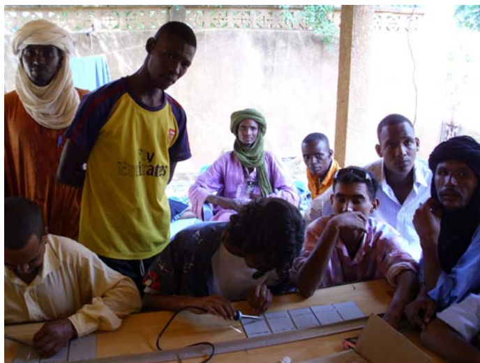
Nomad group learning how to solder PV cells to make a module for a water pump
